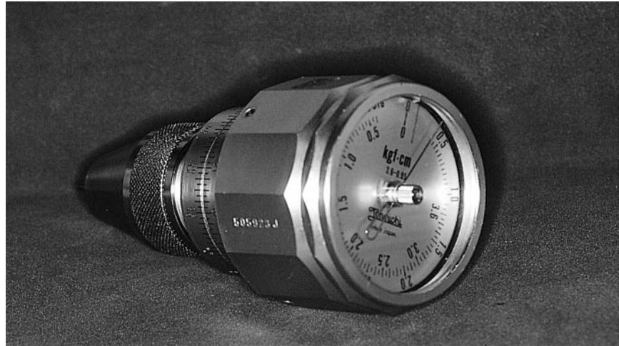
FIGURE 1. Tohnichi torque gauge used for research in Jaarda et al,<sup>5,7</sup> Bakaeen et al,<sup>9</sup> Siamos et al,<sup>10</sup> and Winkler et al (unpublished data, 2003), (Tohnichi America Corporation, Northbrook, Ill).
